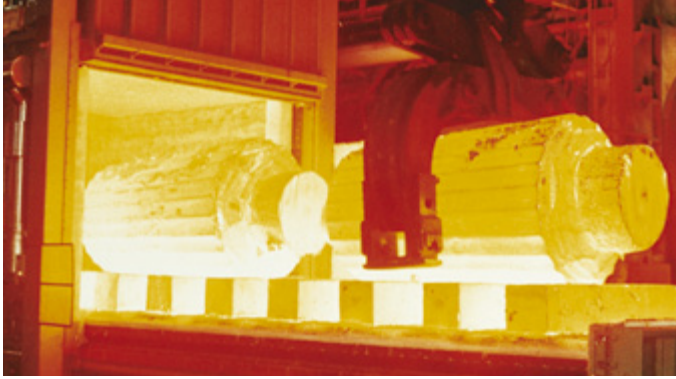
Metallurgical industry: forging furnace
