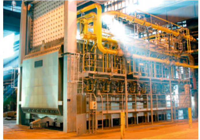
Ceramics industry: intermittent shuttle kiln
