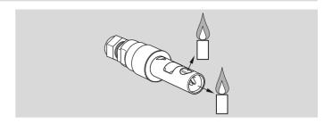
The UV tube can be directed towards the flame from the side or front with the help of the viewing openings in the sensor head.
