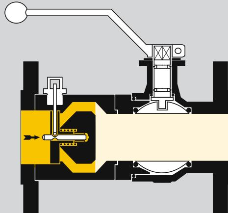
If the ambient temperature increases to more than 95°C in the event of a fire, a seal melts in the thermal equipment trip TAS and releases a spring that is held by a retaining pin. The spring presses the closing taper against the sealing seat ensuring that no more gas can pass through.
