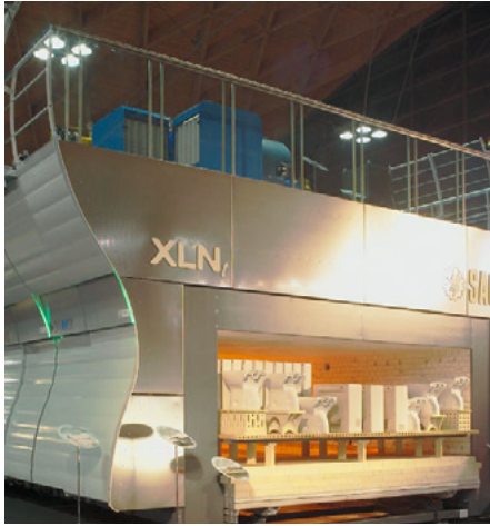
Roller hearth kiln in the ceramics industry
